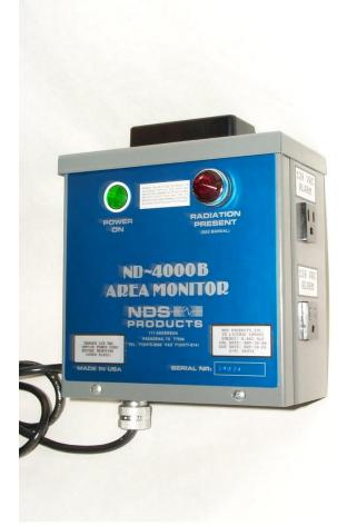
120 VAC hard wired or plug-in economical Area Monitor Non-adjustable trip point at 2 mR/hr Will activate and 120 VAC device such as lights and sirens Two 5 amp 120 VAC remote alarm outlets One AC power On/Off green indicator and one red alarm trip indicator Operating Temperature: -20 to 50 °C (-4 to 122 °F), Humidity: Non-Condensing 95% NEMA 3R steel case: 8" W x 9" H x 5" D 6 pounds Halogen quenched energy compensated GM tube, Gamma and X-Ray from 60-2000 KeV +/- 20%
