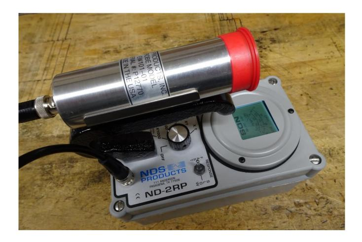
**Dual Detector, Five Range, Thin End Window Survey Meter** LCD Display in Both mR/hr and CPM
