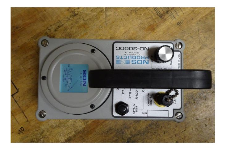
Five Range 0-10 R/hr Dustproof Rugged Survey Meter with built-in dosimeter charger LCD Display available in mR/hr and uSv/hr Two Halogen Quenched Energy Compensated GM Tubes Ranges 0-10,000, 0-1000, 0-100, 0-10, 0-1 mR/hr and 0-100,000, 0-10,000, 0-1000, 0-100, 0-10 uSv/hr Operates on Two ''D'' Cell Batteries
