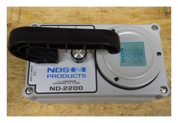
Rugged Dustproof Radiographic Survey Meter Three Ranges 0-1000, 0-100, 0-10 mR/hr or 0-10,000, 0-1000, 0-100 uSv/hr LCD Display available in mr/hr and uSv/hr **Halogen Quenched Energy Compensated GM Tube** Energy Dependence Within 15% from 50-2000 KeV **Fast/Slow Response Switch** Operates on Two "D" Cell Batteries Operating Temperature: -20 to 50 °C (-4 to 122 °F), Humidity: Non-Condensing 95%
