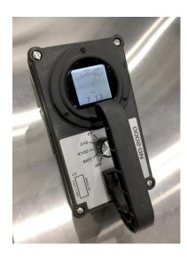
Three Range Dustproof Radiographic Survey Meter Rugged Two Piece Nylon Reinforced Case and Handle LCD Display
