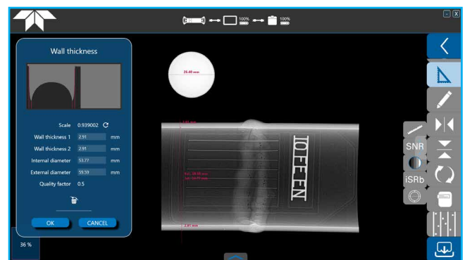
Wall thickness measurement
